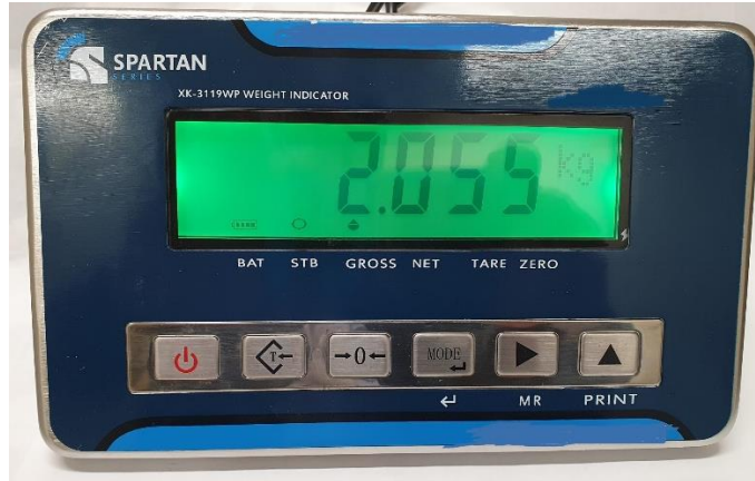
National Weighing Instrument Model Spartan XK3119WP-PRO Weighing Indicator (Pattern)
