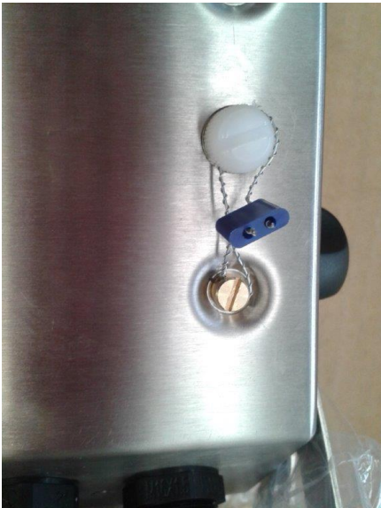
(a) Sealing of Lead and Wire Type
