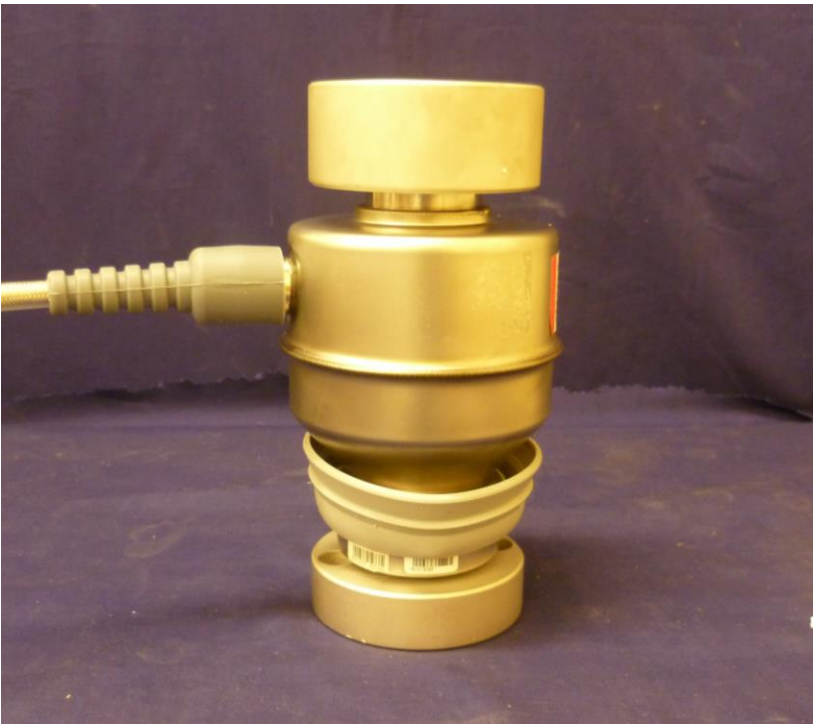
Typical Mounting Arrangement Note: Use without the rubber boot is acceptable.
