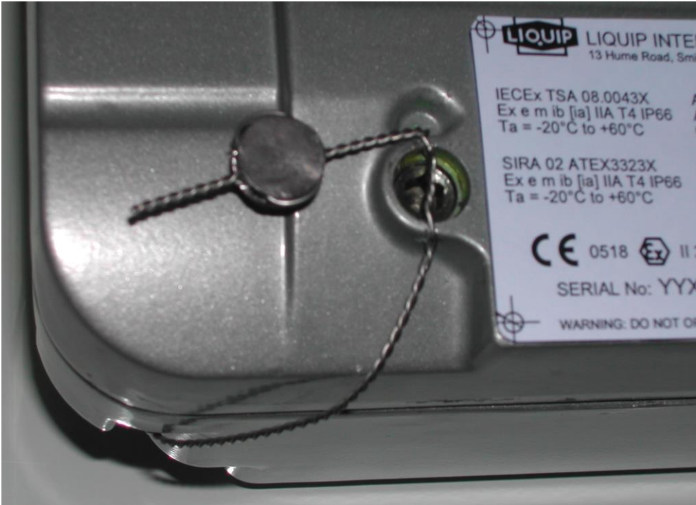
Typical Sealing of the Cal Button to a Cover-mounting Screw (not shown)
