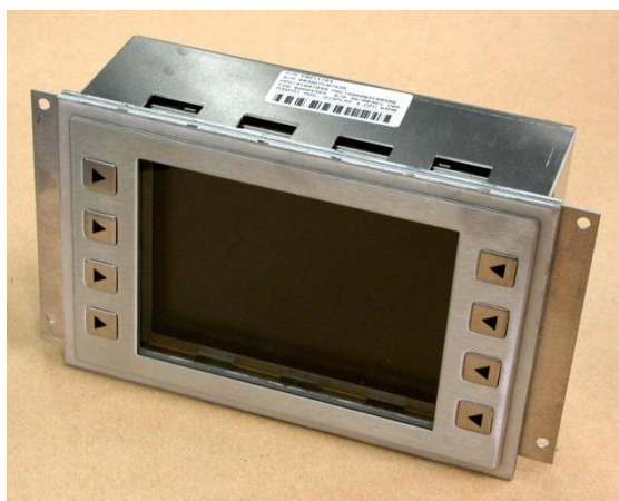
(a) Typical FLEXPAY display unit
