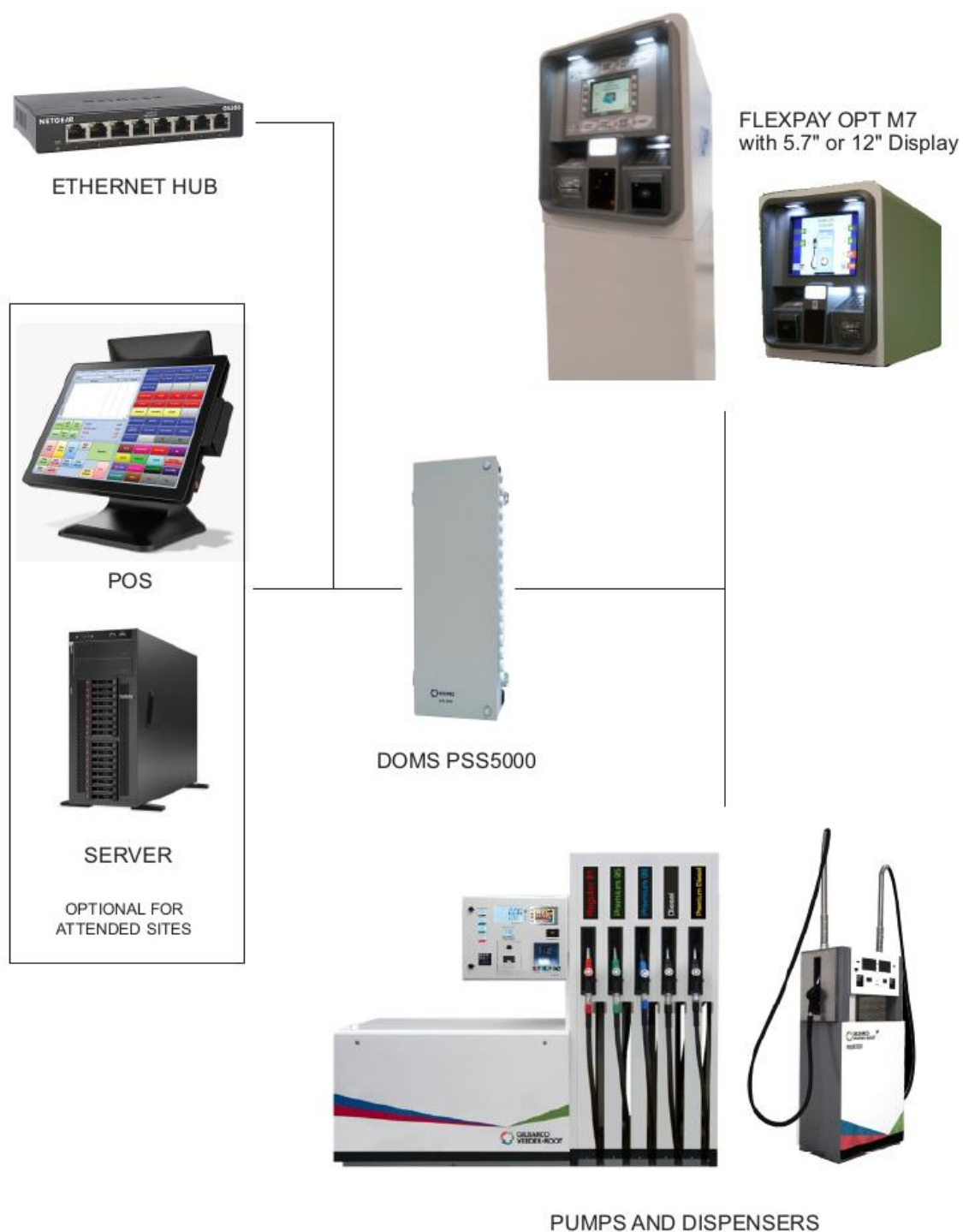
Typical Gilbarco Model FLEXPAY Outdoor Payment Terminal (OPT) M7 With DOMS PSS5000 forecourt controller (variant 4)
