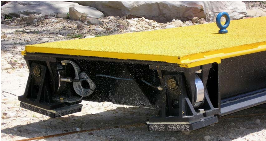
(b) Platform removed, showing load cell mounting arrangement
