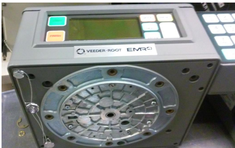
Typical Sealing of the Veeder Root Model EMR4 Meter Mounted Display Head
