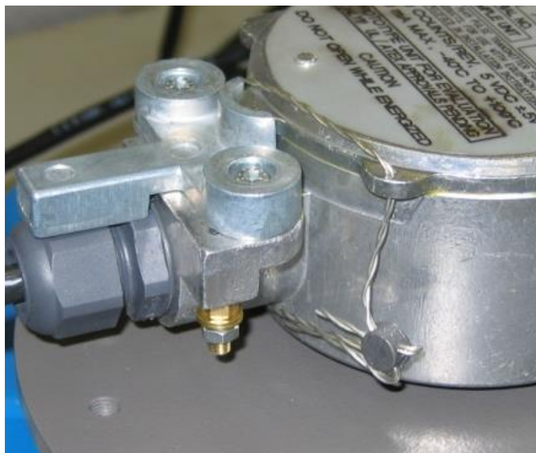
Typical Sealing of the Remote Pulse Transmitter
