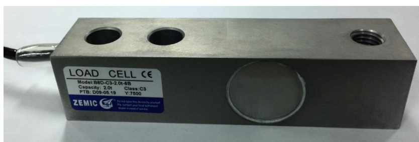
(b) ZEMIC Model B8D Series Load Cell Up to 10 t Maximum Capacity
