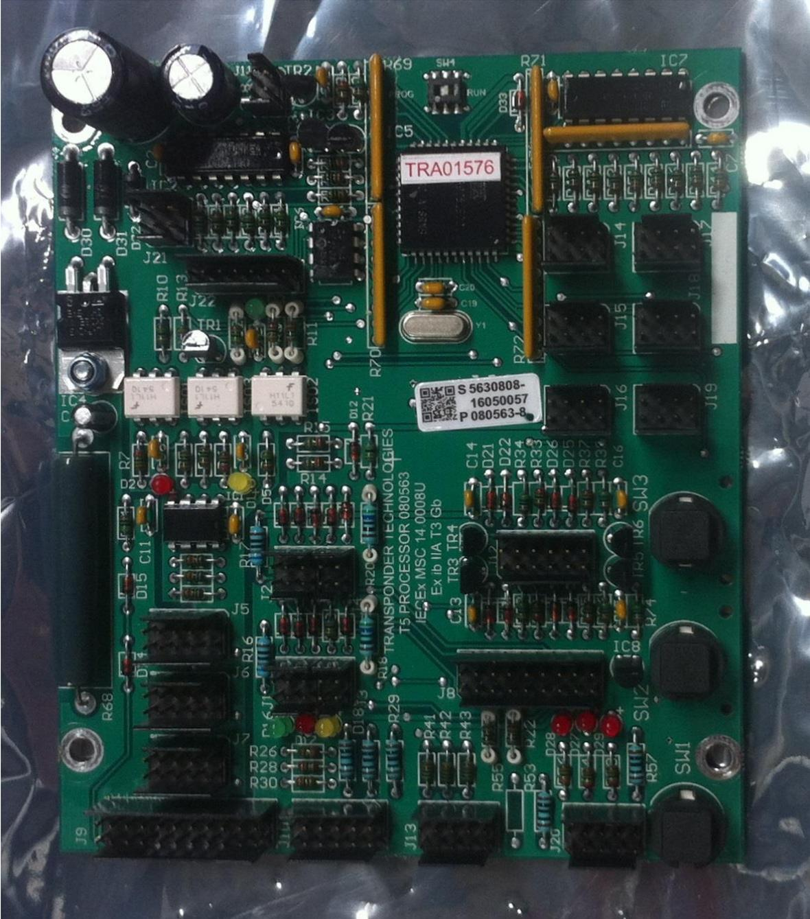
Transponder Technologies Model T5 Calculator/Indicator Processor Board
