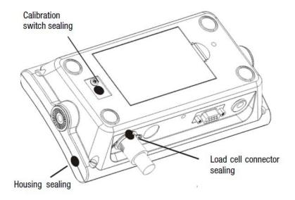
(a) Typical Sealing of PT Model PT252 Digital Indicator (pattern)
