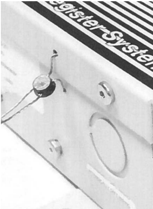
Typical Sealing of the Interconnection Box
