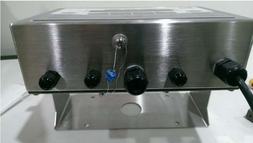
Typical Sealing Using Lead and Wire Type with Drilled Screws
