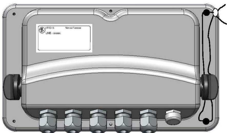
Typical Mechanical Sealing of the Model i20 (pattern) & i30 (variant 1)
