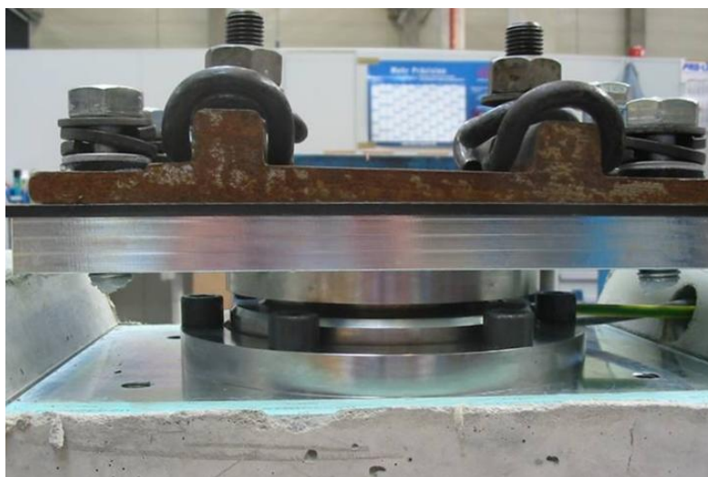
A Typical Mounting Method (in this case for a train weighing in-motion instrument)
