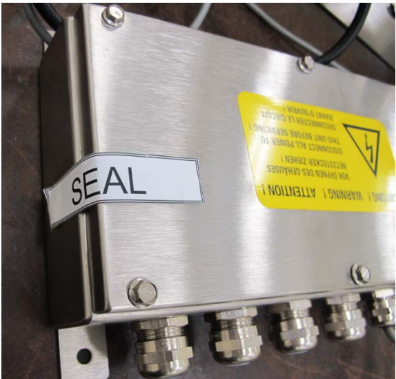
(b) Typical Sealing of Systec Model ADCBox External Scale Multiplexer
