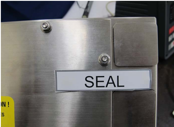
(a) Typical Sealing of Systec Model IT9000E Digital Indicator
