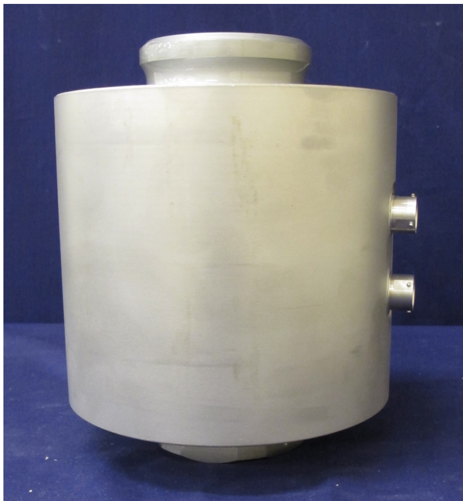
Typical High Capacity SLC820 Series (aka POWERCELL PDX) Load Cell (Variant 2)
