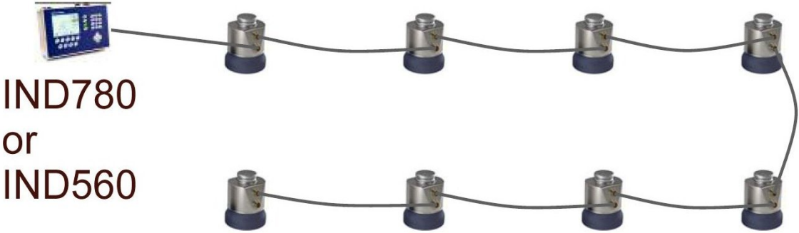
Typical POWERCELL PDX Daisy Chain Network (pattern & variants)
