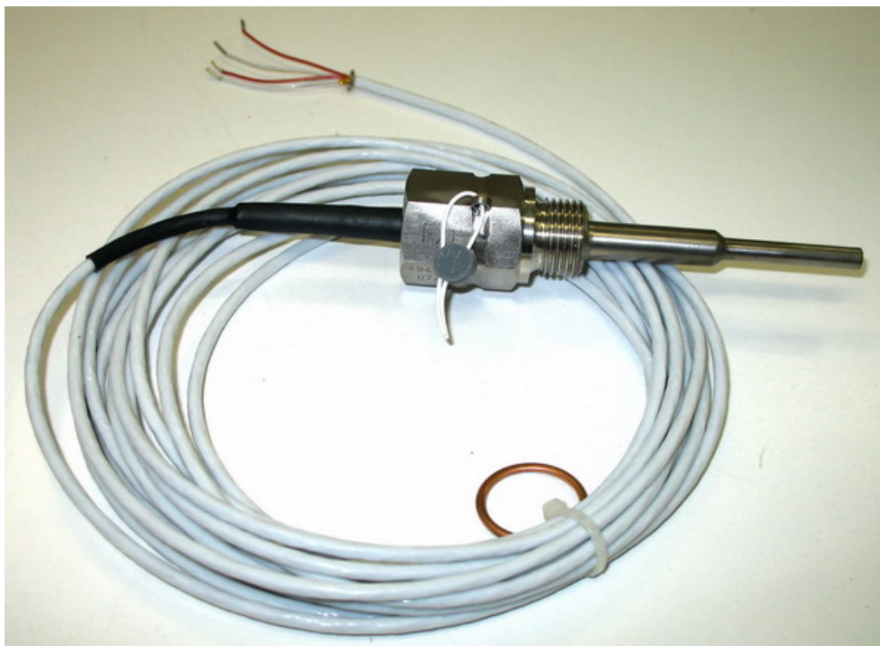
(b) A Typical PT100-Thermometer With Pre-connected Cable
