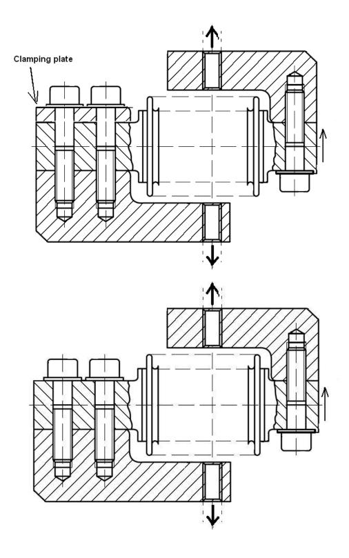
Tension 'Fold back arm' Mounting Arrangements - Variant 2
