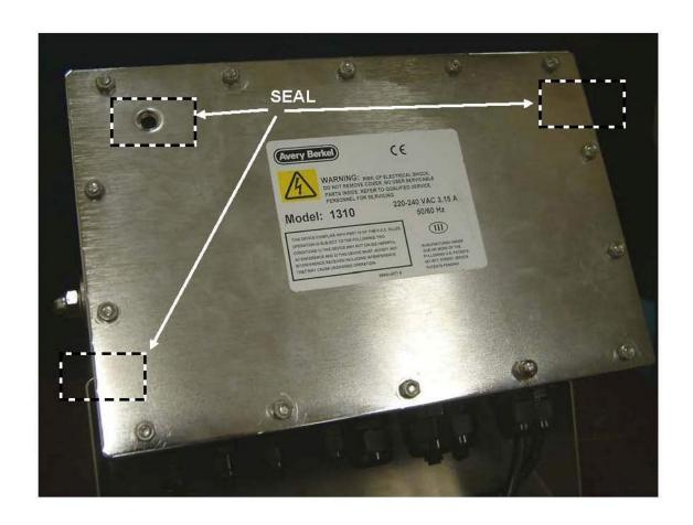
Sealing Arrangement (view from rear of housing)
