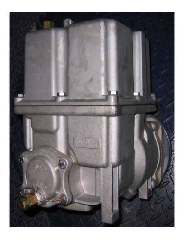
Showing Typical Sealing of Gas Elimination Device Air Test Valve Access Point
