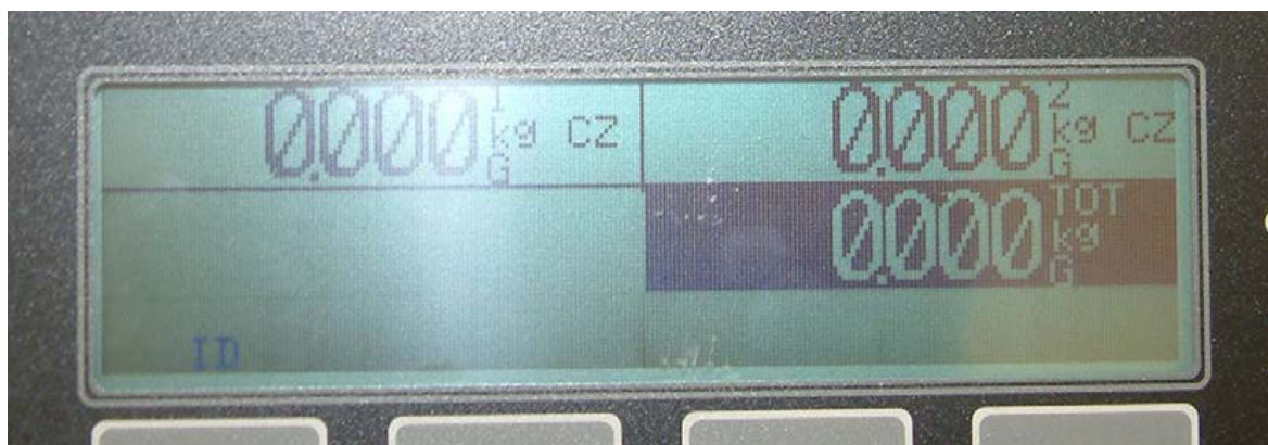
(b) Nuweigh Model JAC 350 Digital Indicator (Variant 7) (aka Cardinal Model 225) – Indication showing summing and 'centre zero' ('CZ') display
