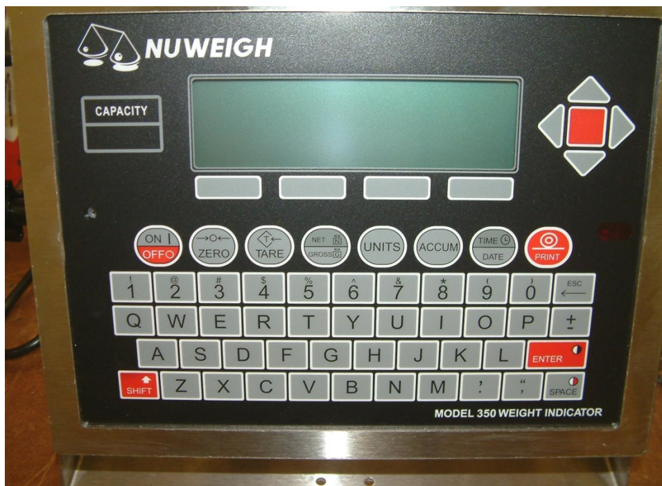
(a) Nuweigh Model JAC 350 Digital Indicator (Variant 7) (aka Cardinal Model 225) – Indicator and keyboard
