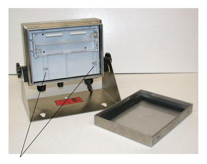
At least one sealing screw to be sealed
