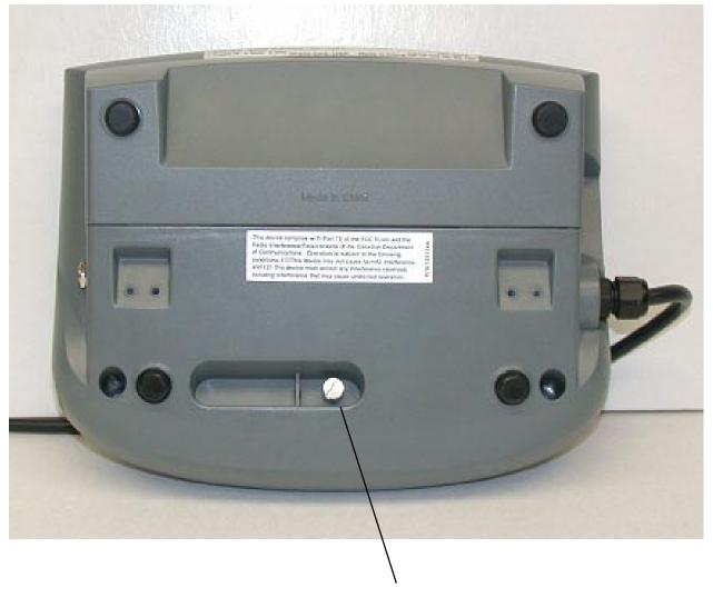
Sealing screw sand fixing for wire and lead seal
