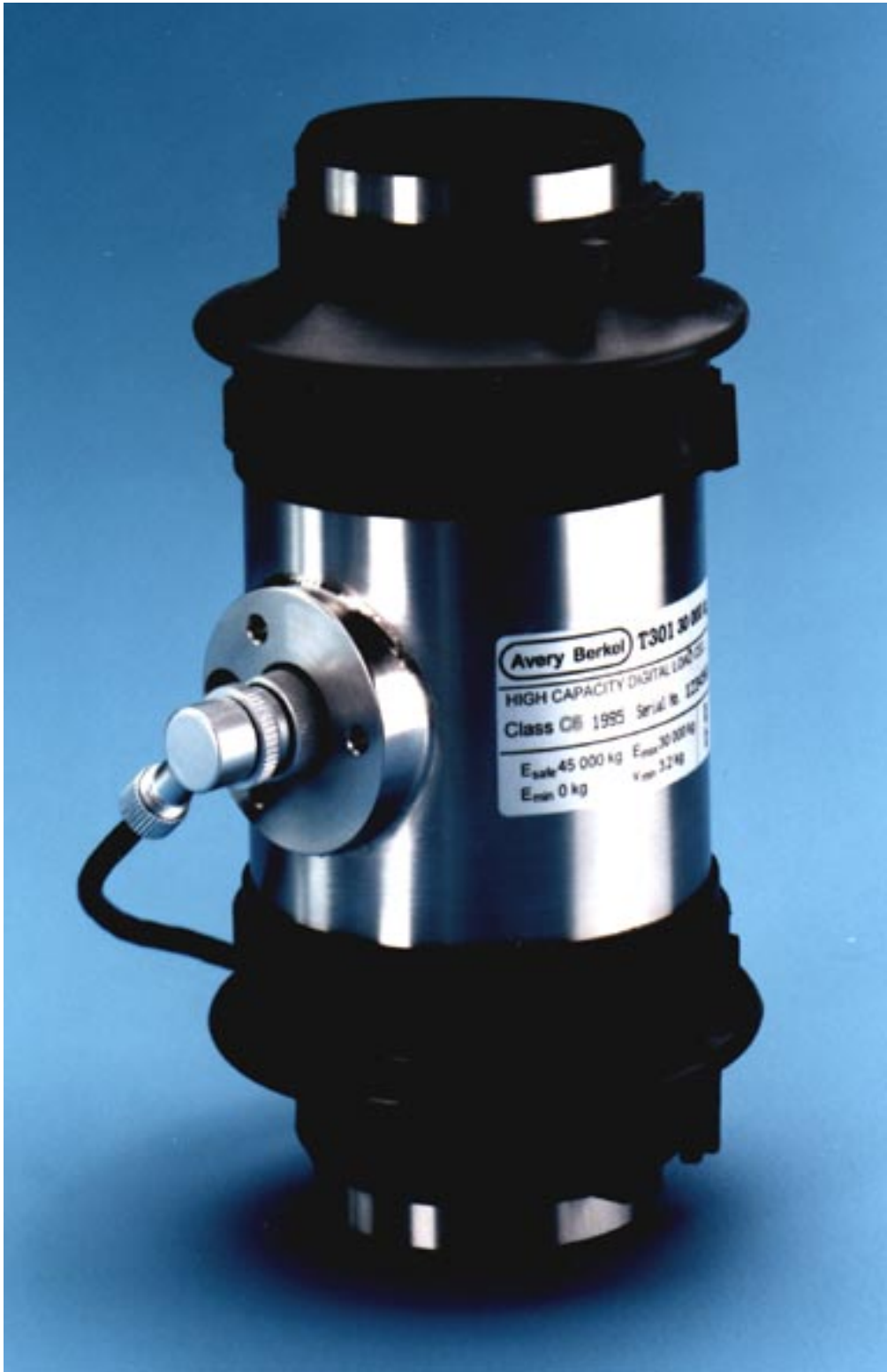
Avery Berkel Model T301 Load Cell With Rubber Bellows Fitted
