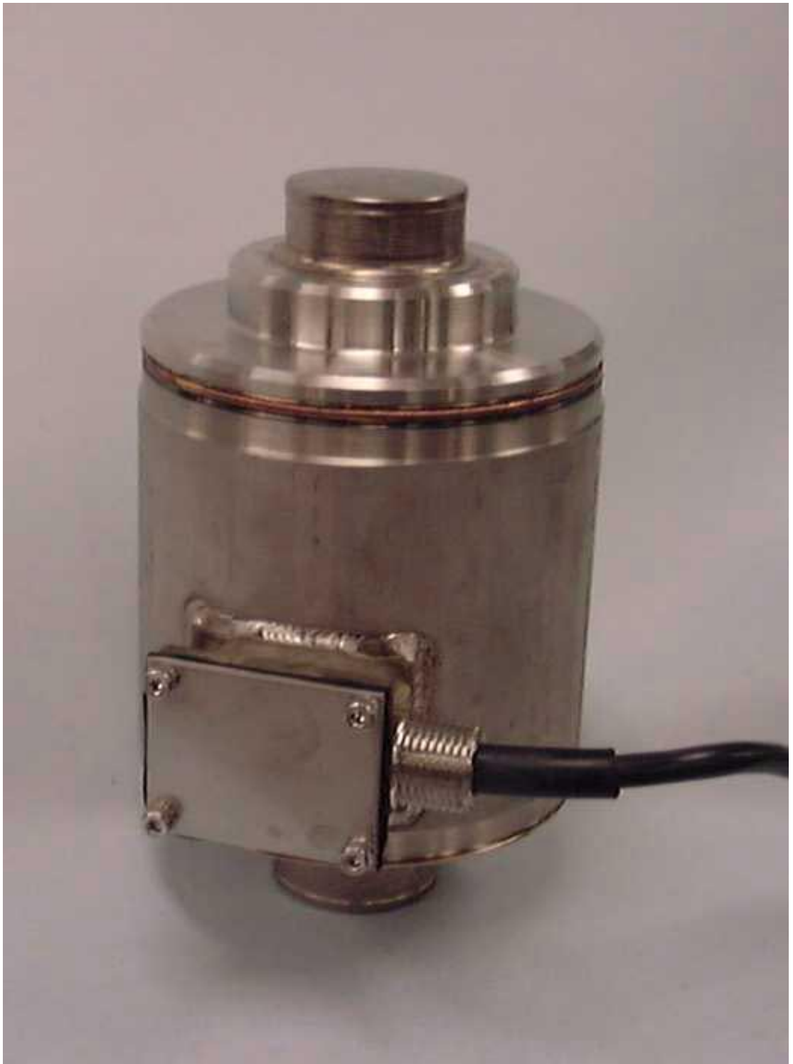
A & D Mercury Model LC2226-T030 Load Cell
