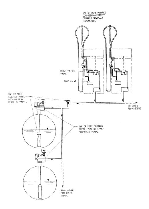
Schematic Diagram Of A Typical STP System
