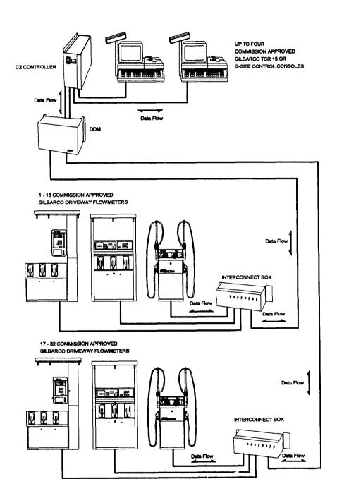
Schematic Diagram of a Typical Gilbarco Model TMS-15 System
