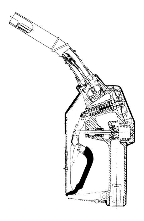
Schematic Of 11A Series Nozzle
