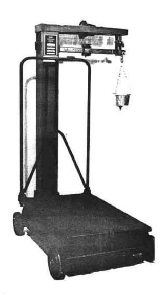
Avery Counting and Weighing Machine Model 3901 AAG — with Counting Ratio 100 : 1
