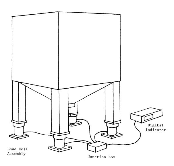
Toledo Model 2375 Hopper Weighing Instrument
