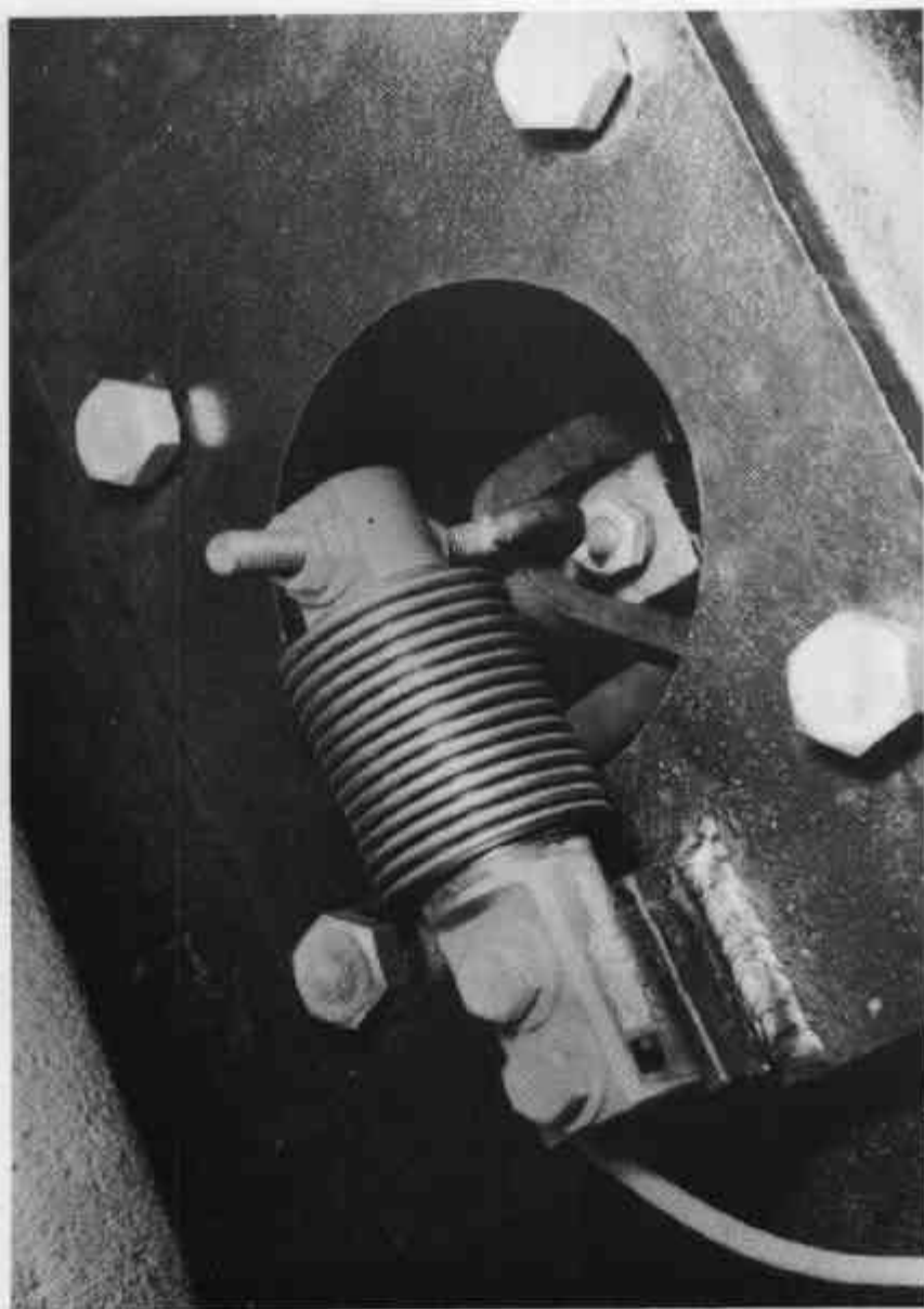
Load Cell, Pullrod, and Attachment of Load Cell to Weighing Unit
