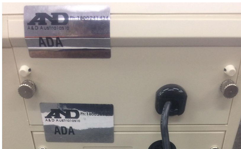
(b) Destructible Adhesive Labels Sealing Arrangement
