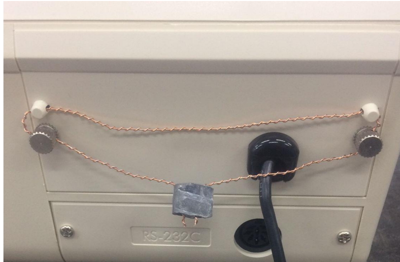
(a) Lead and Wire Type Sealing Arrangement
