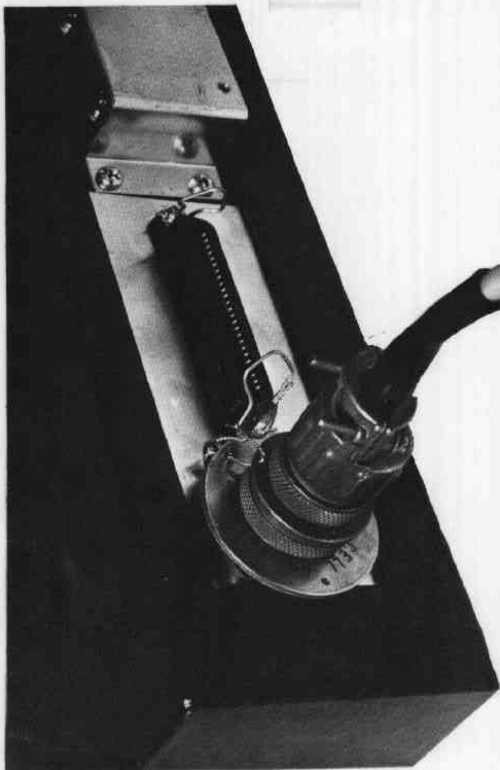
Sealing — Load Cell Cable and Serial Number
