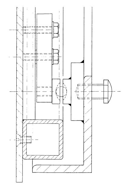
Showing P3000 Load Cell Mounting
