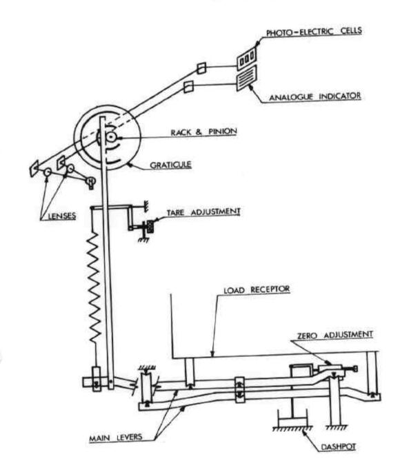
Levers and Optical-projection System — Schematic Diagram 29/1/75
