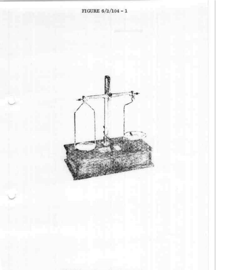
Wedderburn Dispensing Beam-scale
