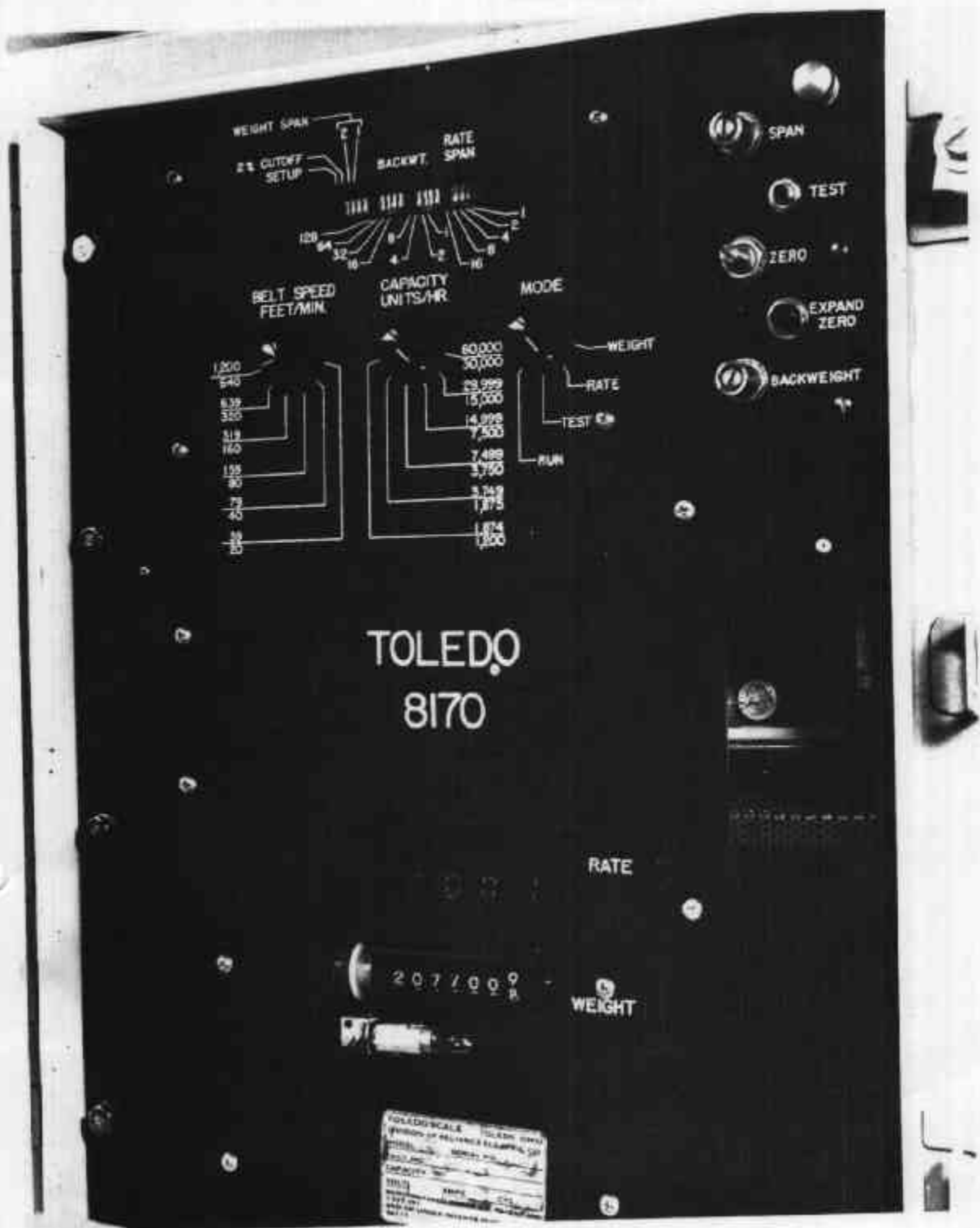
Computing and Totalizing Unit — Calibration of Zero Adjustments
