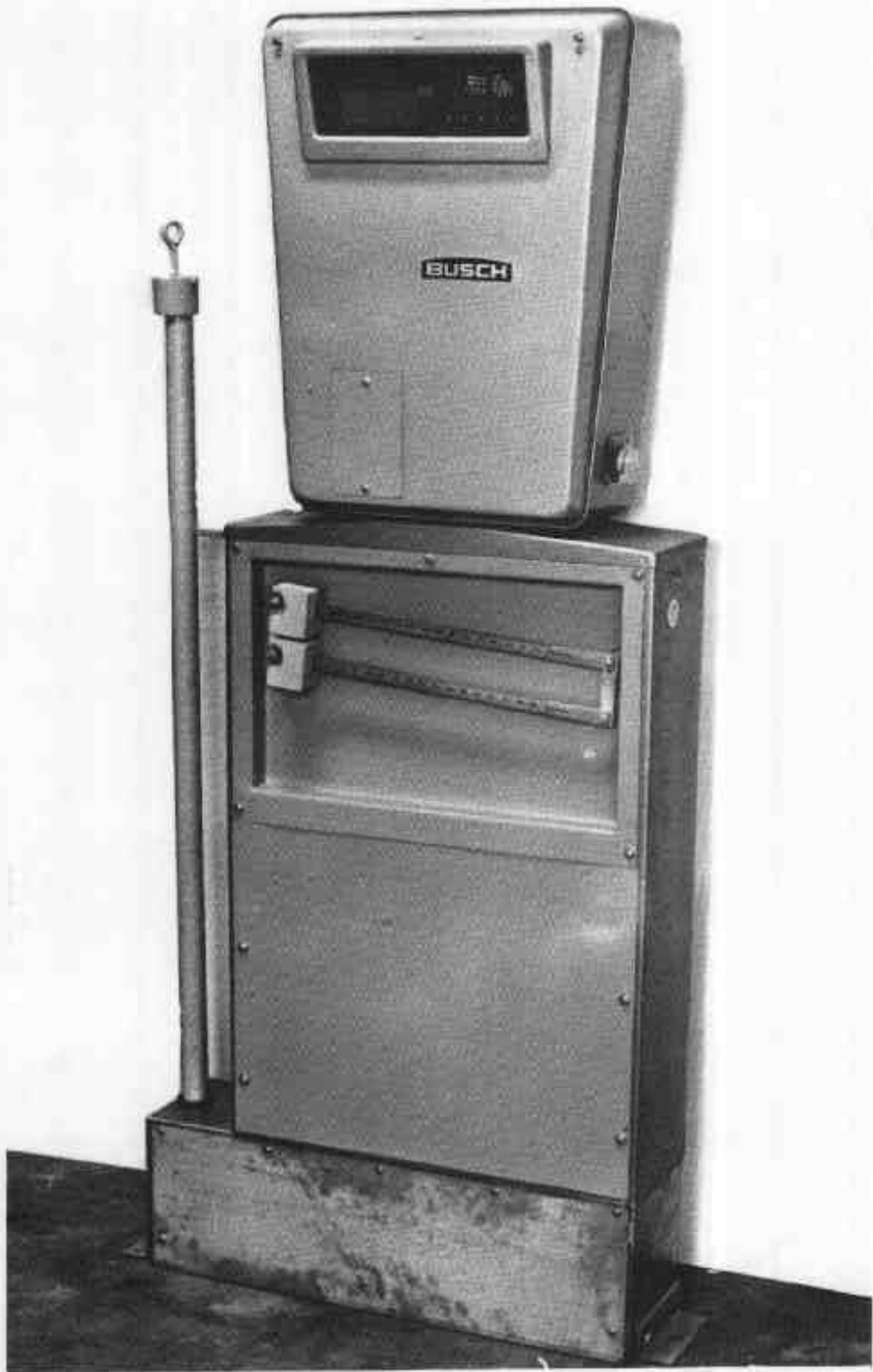
Headwork with External Tare Bars
