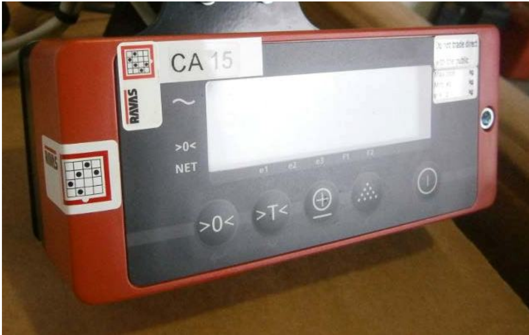
(a) Sealing of Indicator Using Destructible Adhesive Label/s
