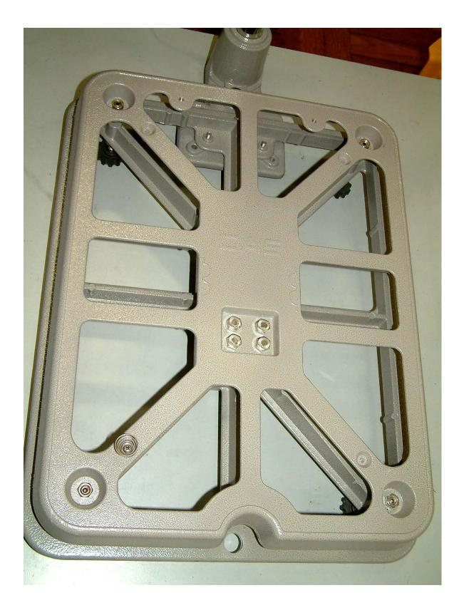
CAS Model BW-1N (BW-60RB) basework (platter removed)
