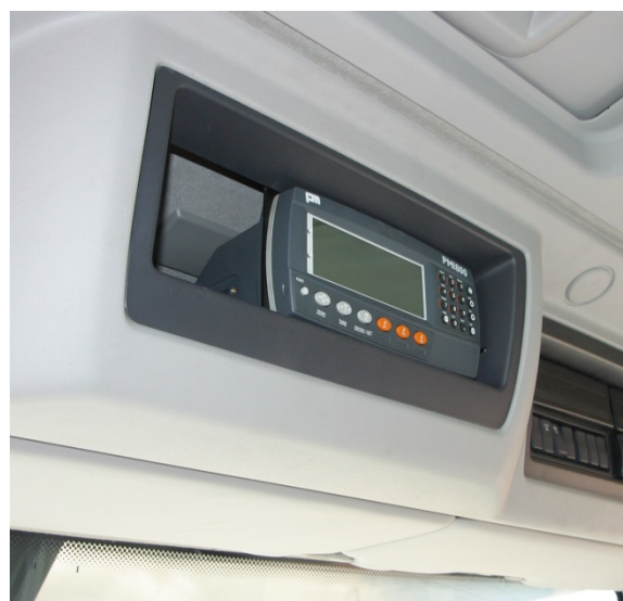
(b) PM Onboard Model PM1800 Indicator including Installation on a Typical Vehicle
