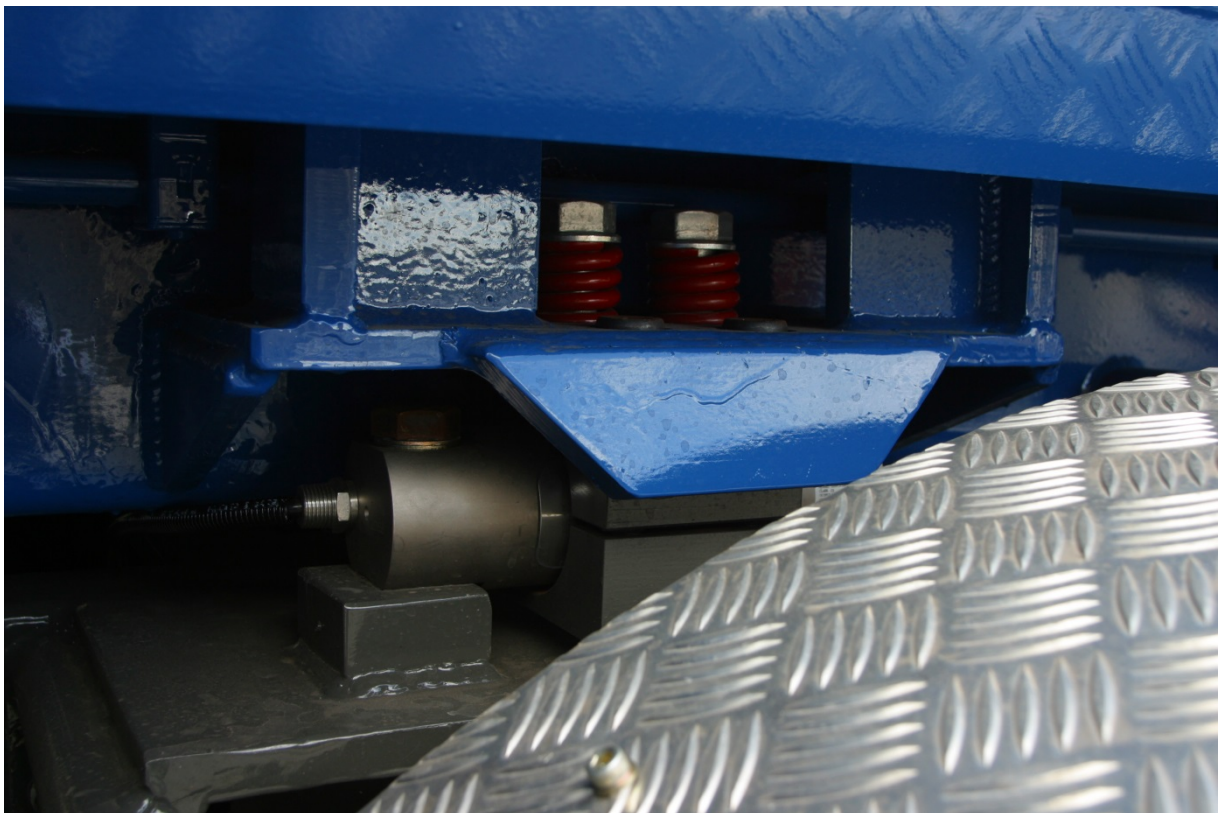
Revere Transducers Inc Model 5103 C3-50K-9B Load Cell with Typical Mounting Arrangements
