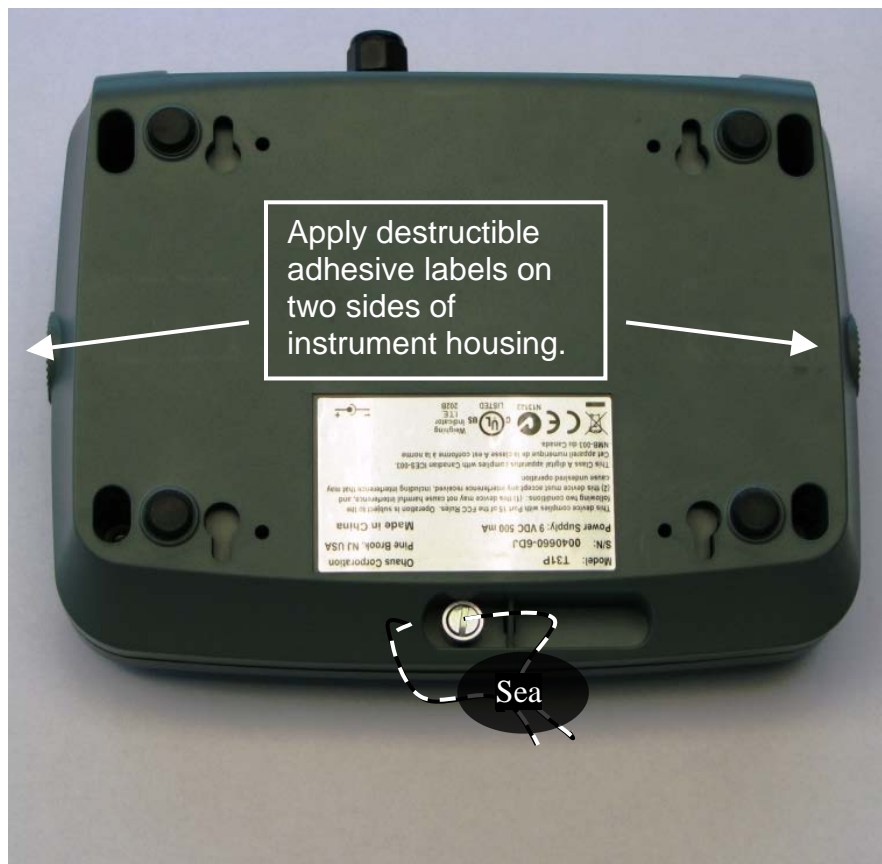
(b) Sealing of Ohaus T31PAU (lead and wire type seal, or labels)
