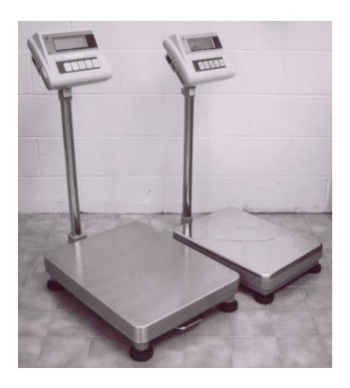
Excell Model LRW and MRW Weighing Instruments
