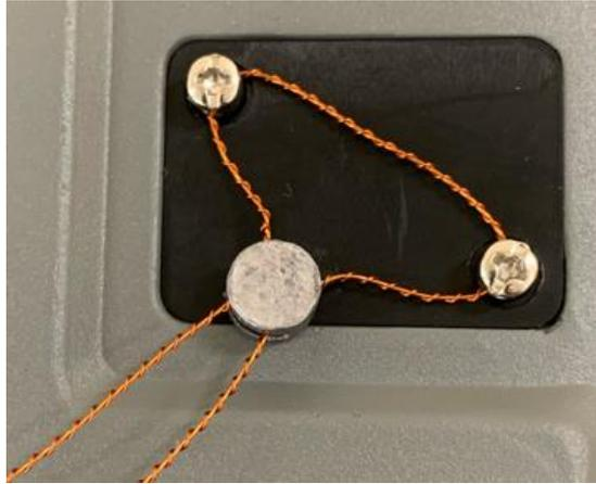
(a) Sealing of Lead and Wire Type with Drilled Screws
