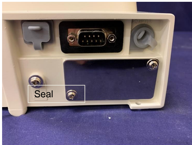
(b) Sealing Arrangement Using Destructible Adhesive Label
