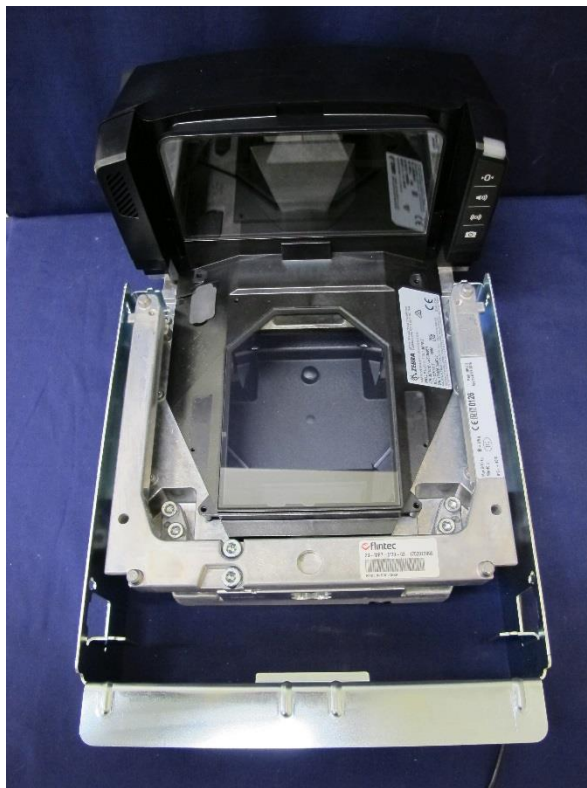
(b) NCR Model MP7001 Weighing Instrument With Load Receptor Plate Removed (Pattern)
