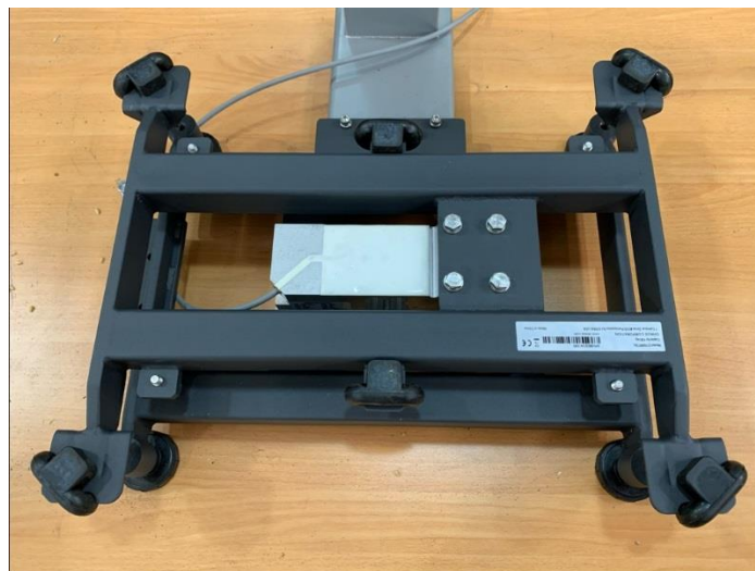
(b) Ohaus Model D52P Series Basework Fitted with a Mettler Toledo 0805 Load Cell
