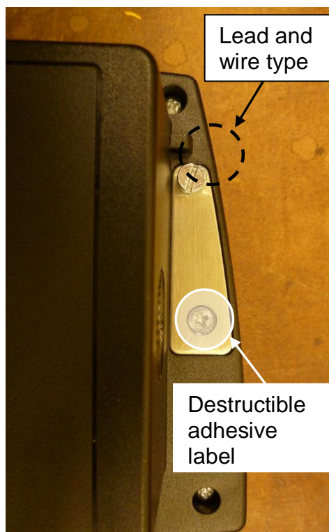
(b) Sealing of TD52P Digital Indicator
