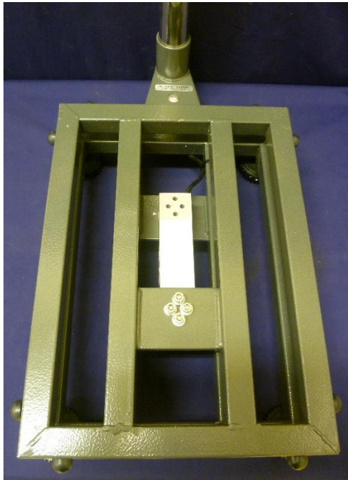
(a) Wedderburn Model WS209 Weighing Instrument Fitted with a Zemic L6E or Mavin NA1 or Mavin NA2 Load Cell
