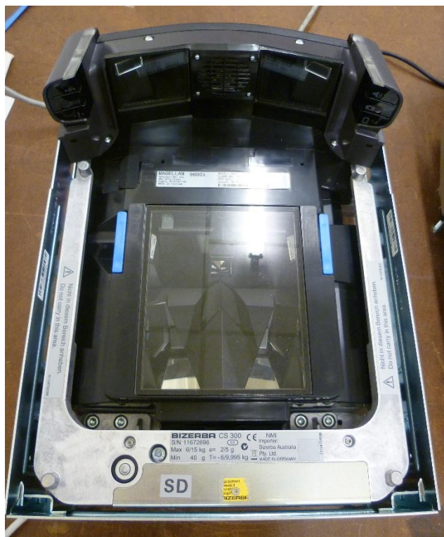
(b) Bizerba Model CS300MA98 With Load Receptor Plate Removed (Pattern)
