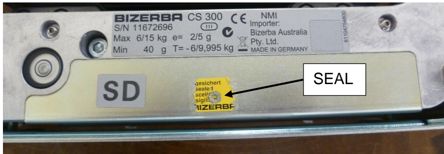
(a) Sealing of Model CS300MA98
