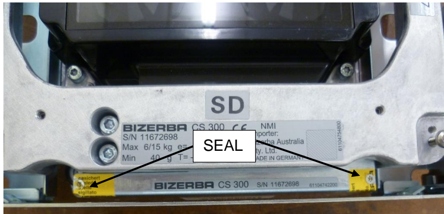
(b) Sealing of Model CS300MA94
