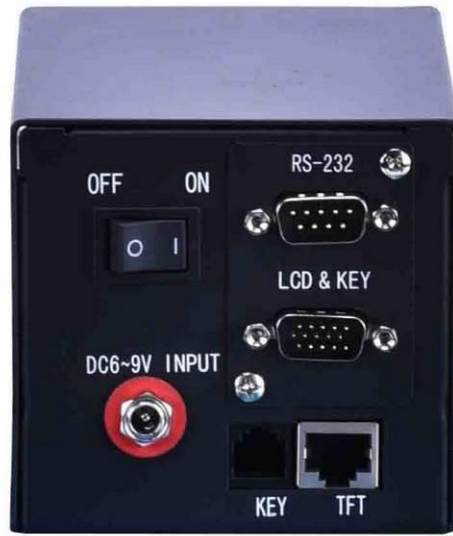
Front View of External Control Box
