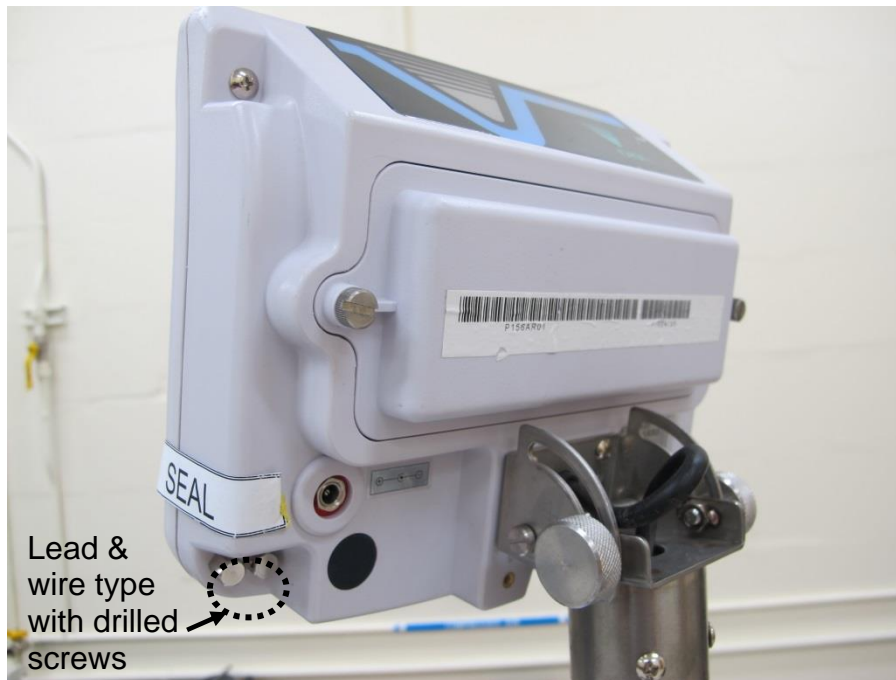
(b) Typical Sealing of Model Digi DS-531 Weighing Instruments
